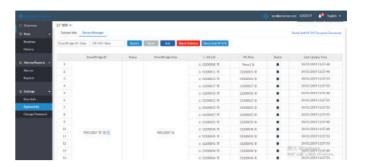
2. Input the microinverter IDs which need to be added to the template. On the left side of the following template is the EnverBridge ID, and on the right side is the microinverter ID.
